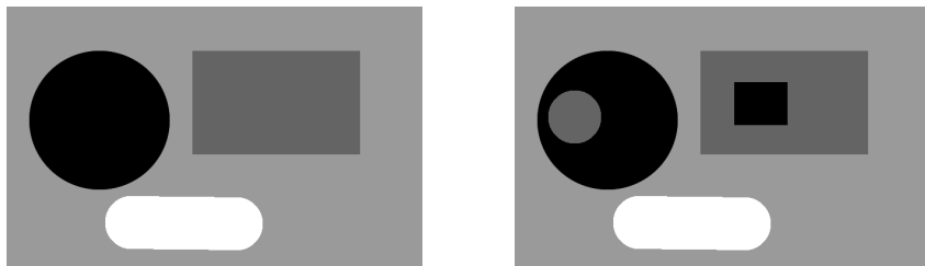
Figure 1: Example of an \alpha - \beta -swap move. The labeling on the right is a “dark gray”-“black”-swap move from the labeling on the left.
